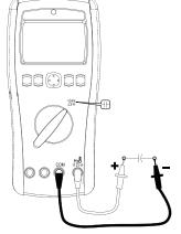
The ranges of measuring capacitance are 40nF, 400nF, 4uF, 40uF, 400uF, 4mF and 40mF.
