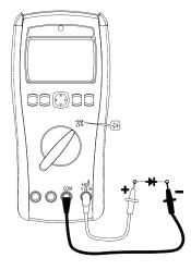
Use the diode function to check diodes, transistors, silicon controlled rectifiers (SCRs), and other semiconductor devices. This function tests a semiconductor junction by sending a current through the junction, then measuring the junction's voltage drop. A good silicon junction drops between 0.5V and 0.8V.
