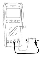
The ranges of measuring resistance are  $400\Omega$ ,  $4k\Omega$ ,  $40k\Omega$ ,  $400k\Omega$ ,  $4M\Omega$ , and  $40M\Omega$ .
