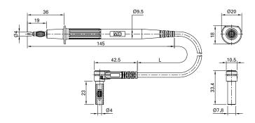
Highly flexible, with insulation in silicone. One end with  $\varnothing$  4 mm test probe with spring-loaded MULTILAM, the other end with right angled  $\varnothing$  4 mm MULTILAM plug with rigid insulating sleeve. Supplied with protective cap.
