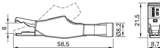
Test clip with all-round insulation. Toothed gripping jaws with fine-wire clamping surface.
