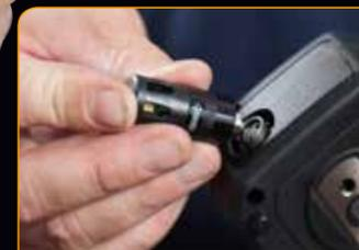
Field Replaceable T/RH Sensor
